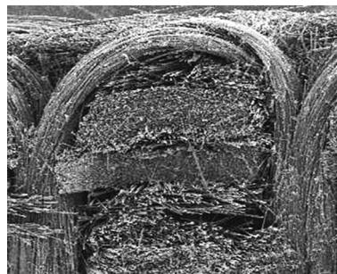
图2 Tufting缝合预制体结构 Fig.2 Structure of tufting preform
